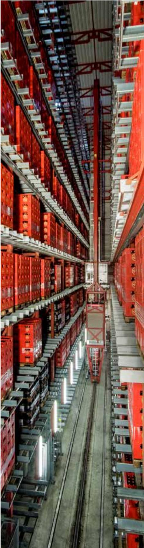
principle (first in first out) is not applicable to large beverage batches. So they are ideal for deep storage channels, which provide high storage density for maximum capacity on minimum floorspace.
